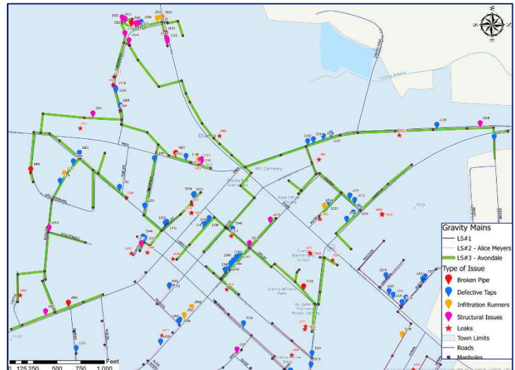
Figure 1 – Map of I&I Issues Identified (Lift Station #3)
