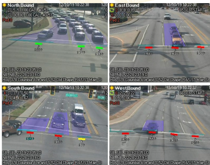
The cameras which feed information into Lexington’s Adaptive Signalization System are mounted alongside the town’s traffic lights. Photo: Town of Lexington.
